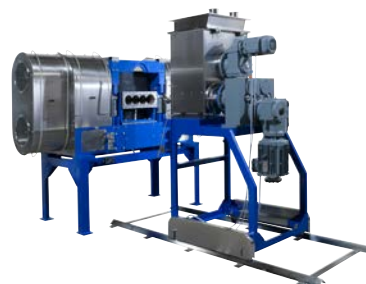
PP 175 Throughput up to 500 kg/h Variable number of screws: 1, 2 or 4 As standard with the patented Combi-Vent-Feeder® Option: Cooled rollers
