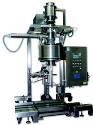
Mobile endless-foil filling station with Vibro-Dos®
