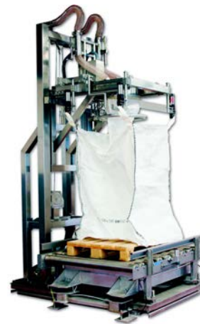
Big-Bag filling with conveyor and product compression
